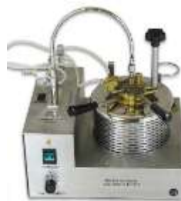
Fig 2.4: Pensky-marten Flash Point Tester [13]
